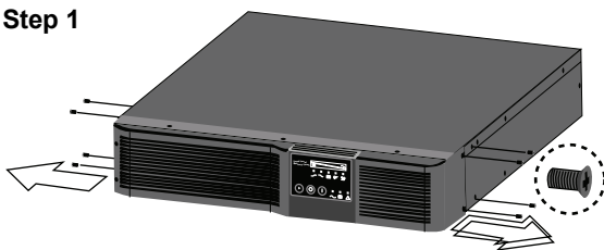
Figure 8 Convert the Liebert PSI XR for rack installation
